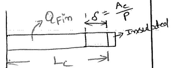
→ Fins subjected to ~~at their tip~~ <sup>tip</sup> convection at their tips can be treated as fins with insulated tip by replacing the actual fin length by the corrected length ( $L_c$ )
