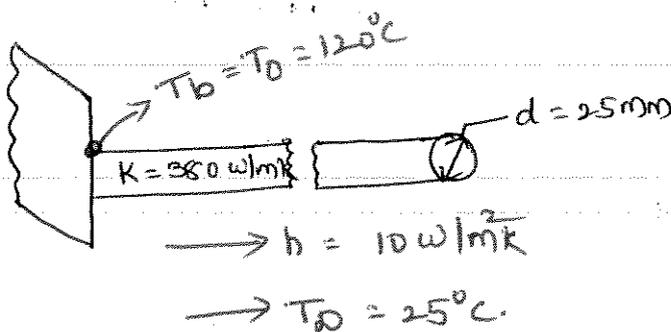
1) The heat loss from the ~~fin~~ infinite long fin
