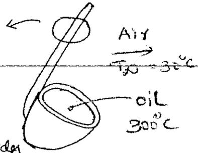
$$\frac{T(x) - T_0}{T_0 - T_{\infty}} = e^{-mx}$$
