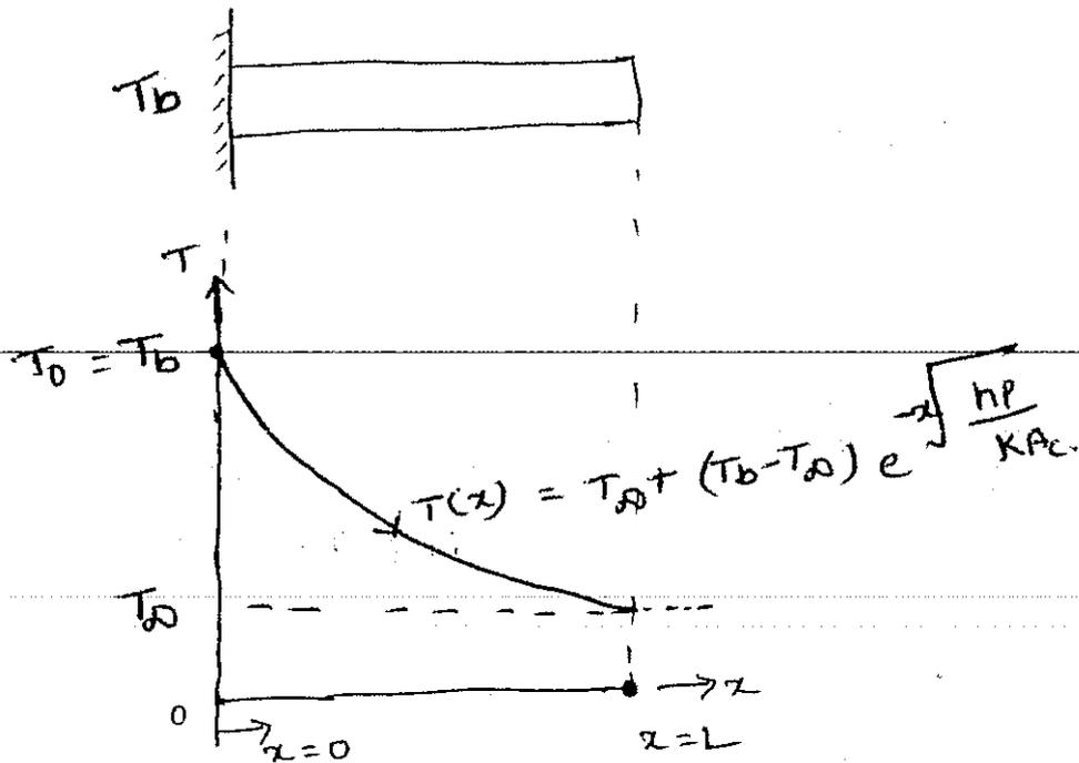
→ for sufficiently long fin of uniform cross section ( $A_c = \text{const}$ ) the temperature of fin at the fin tip approaches the specified temperature  $T_{\infty}$  and thus  $\theta$  approaches zero.
