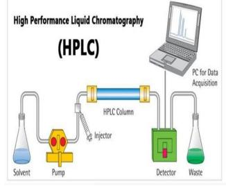
• Most pumps used in current LC systems generate the flow by back-and-forth motion of a motor-driven piston (reciprocating pumps). Because of this piston motion, it produces "pulses".
