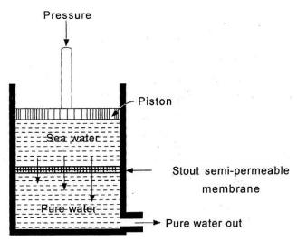
**Method of purification:** The reverse osmosis cell consists of a chamber fitted with a semi permeable membrane, above which sea water / impure water is taken and a pressure of 15 to 40  $kg/cm^2$  is applied on the sea water/impure water. The pure water is forced through the semi permeable membrane which is made of very thin films of cellulose acetate. However, superior membrane made of polymethylmethacrylate and polyamide polymers have come to use.
